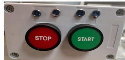
Fig. 4. Start/Stop pushbuttons and LED indicators.
